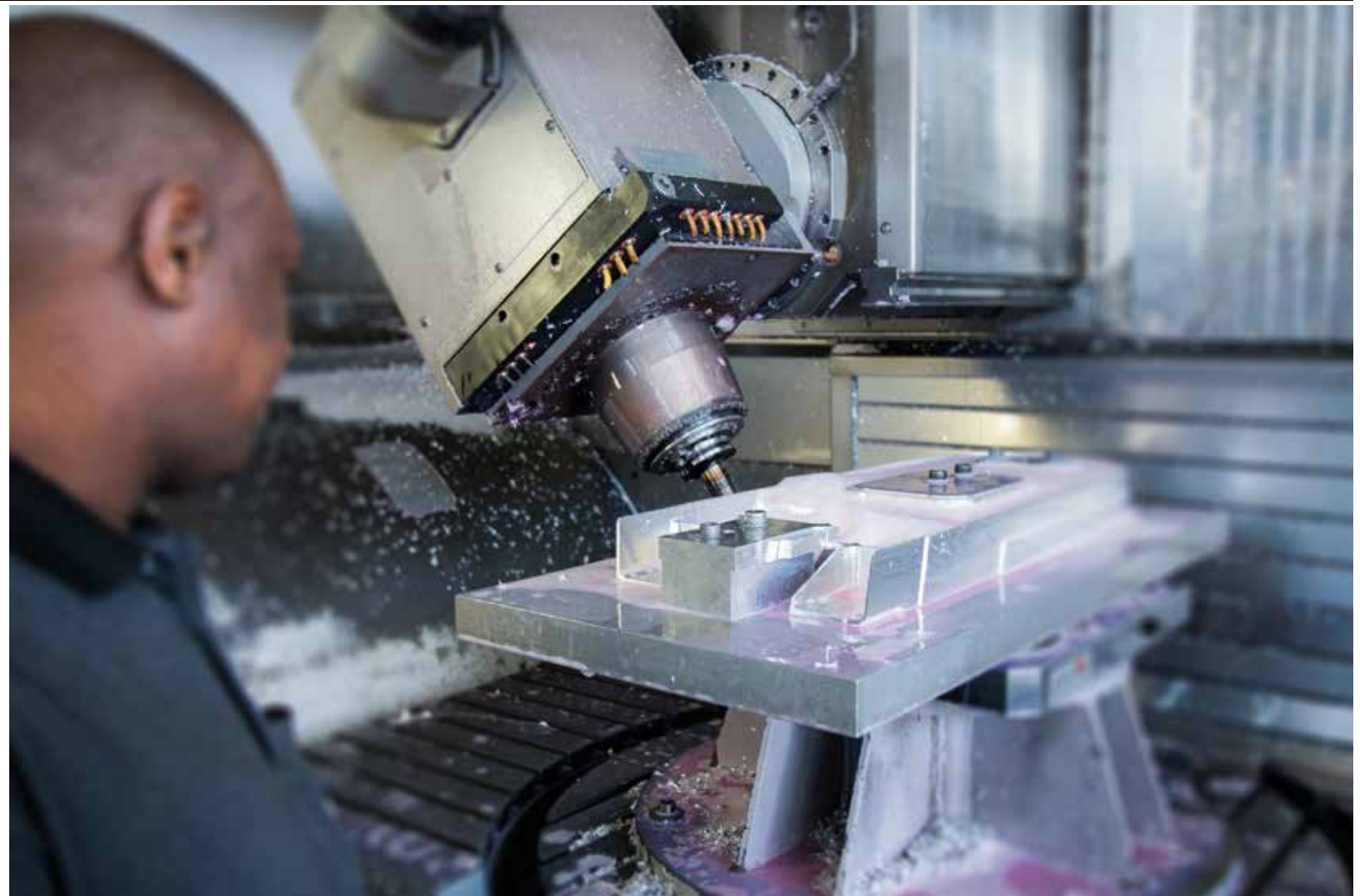
Creating high-tech jobs: a computer controlled cutting machine is used to cut aluminum aircraft components for the global aerospace industry.
